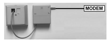
Note: the left located RJ11 jack of the NTP can also be used for a PSTN telephone in absence of VDSL service.
